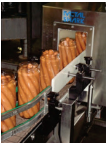
BD with High Pressure Wash down in Meat Production Line
