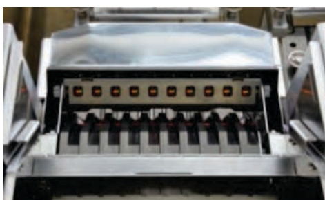
Fail-safe design with rejection confirmation sensor
