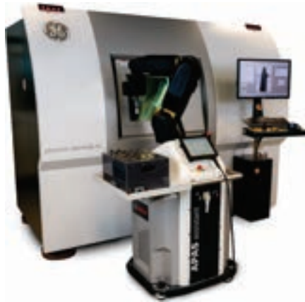
GE Phoenix v|tome|x m with robot 3D X-Ray CT for Analysis and Metrology
