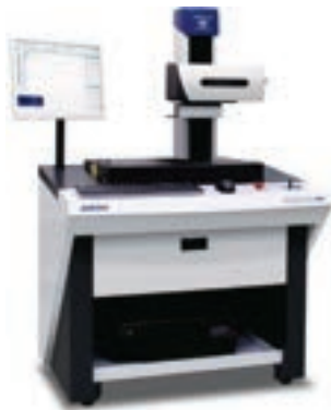
Accretech Surfcom NEX 2-in-1 Roughness/Contour Tester
