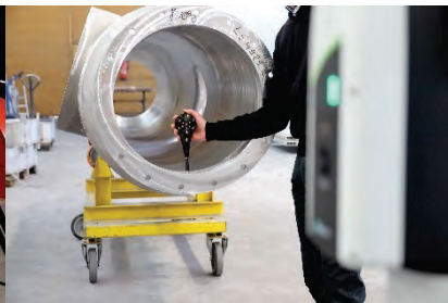
Mounting Hole Location Check
