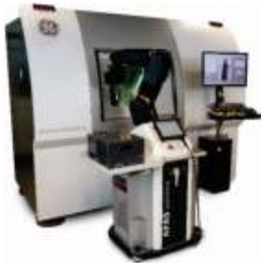
GE Phoenix v|tome|m with robot 3D X-Ray CT for Analysis and Metrology
