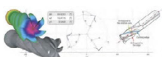
Angle Measurement – Measure clearance/wedge/rake angles of inserts, drills, end mills and other round tools.
