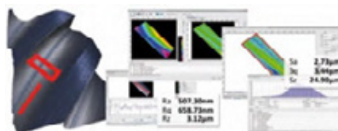
Tool Roughness Measurement – Measure tool roughness both profile and areal based in addition to chipping along the edge
