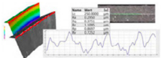
Chipping Measurement – High res measurement of ISO 4287 parameters ( R_a , R_q , R_z , R_p , R_v ) to view defects along edge
