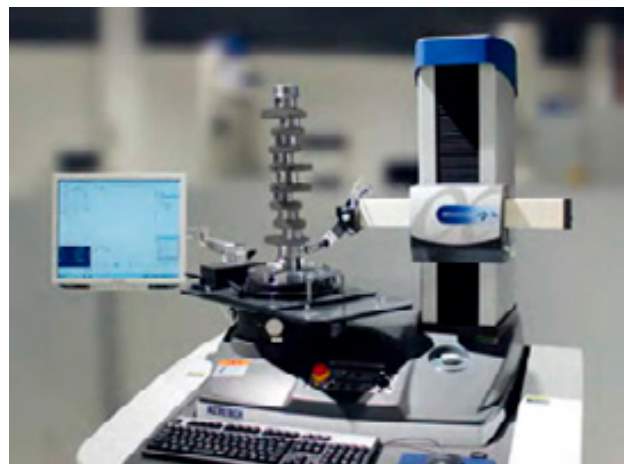
Measuring crankshaft using designated jig tool
