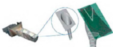
Automatic Measurement of Cooling Holes – Automatically verifying angle, size, and shape of up to 500 cooling holes, some of them with different shapes
