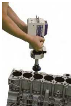
Replaceable Stylus for diameter differences up to 25mm
