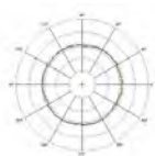
Rotation accuracy 0.06 \mu m at 4/min rotational speed
