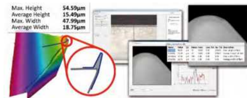
Flash (Burr) Measurement – Flash Width and Height to predict potential wear of molding tools in inserts
