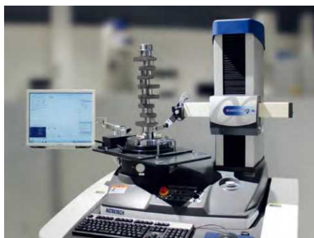
Measuring crankshaft using designated jig tool
