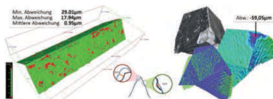
Form Deviation with Difference Measurement – 3D measurements compared to CAD with min/max/mean deviations visualised graphically in colour
