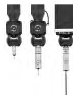
Extension bars; Autojoint fitting \varnothing 25mm with connection repeatability: 1 \mu m at stylus tip, 50mm from autojoint
